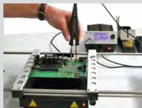
IRHP 200 infrared rework heating plate to assist in the soldering and desoldering process on multilayer boards or high-mass components
