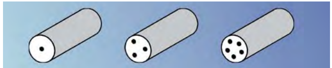
Solder wire with one or with multiple flux cores
